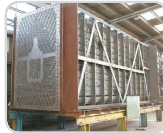
Condenser for nuclear plant
